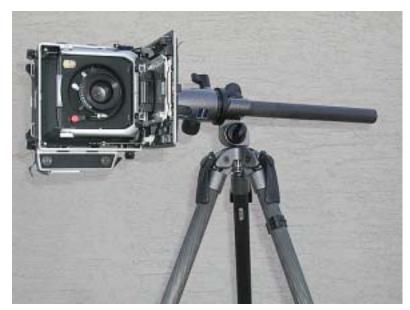
Linhof 4x5 mounted sideways and Vertically on the tripod. This setup is not necessary to take a vertical photograph thanks to the rotating back. However, it can be useful in certain occasions, such as with wide angle lenses when using the drop bed feature (needed to avoid having the bed in the photograph) is not practical.
