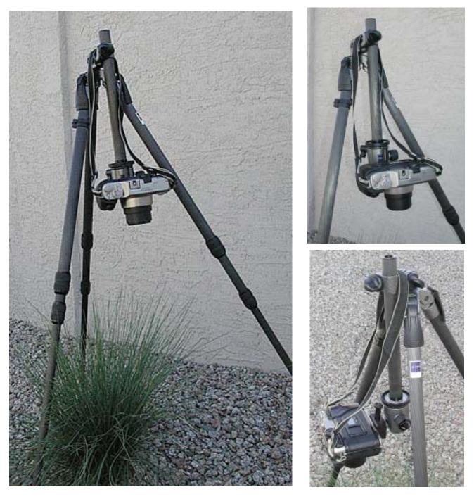
The Fuji 645 zi mounted sideways and downward. The ideal setup to photograph close ups of elements on the ground. Note that the tripod can be positioned closer to the ground simply by not extending the legs as much as I did. Make sure the camera shoulder strap is not in the frame!
