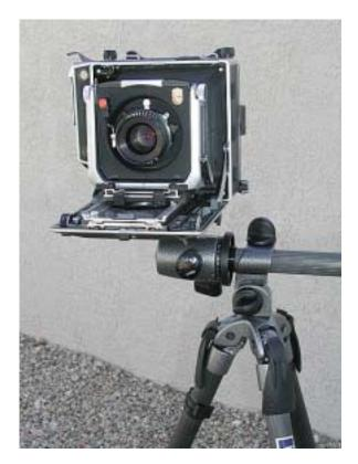
Linhof 4x5 mounted sideways and vertically on the tripod. Since the Linhof has a rotating back it is possible to take both vertical and horizontal view with this setup.
