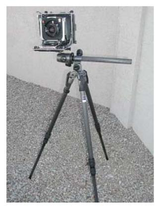
Linhof Master Teknica on sideways center column. Since the center of gravity is only off a couple inches from the actual center of the tripod this configuration is actually quite rigid and vibration free.
